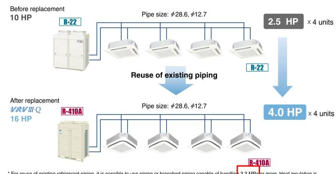
\* For reuse of existing refrigerant piping, it is possible to use piping or branched piping capable of handling 3.3 MPa or more. Heat insulation is necessary for liquid piping and gas piping.
